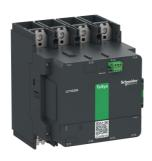
High power contactor, TeSys Giga, 4 pole (4NO), AC-1 <=440V 385A, standard version, 48...130V wide band AC/DC coil
